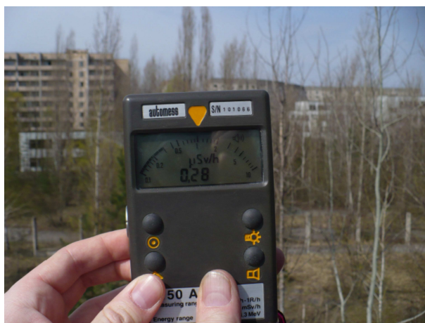
FIGURE 2. Measuring radiation on April 10, 2008 at a sport stadium downtown of Pripjat, about 4 km NW from Chernobyl reactor. The dose rate was 0.28 \mu\text{Sv/h} (2.5 mSv/year). Based on Fornalski (2009).
